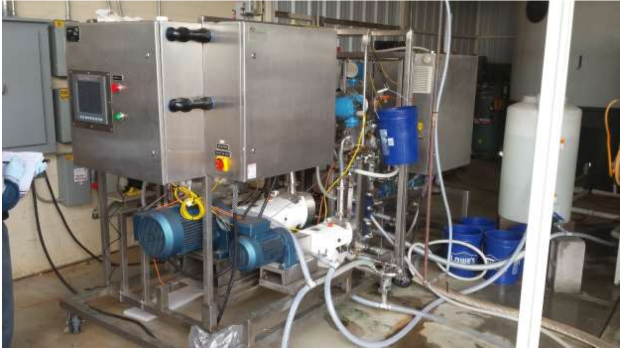
Figure 1. Photo of the Phase II continuous flow pilot scale algae dewatering skid
