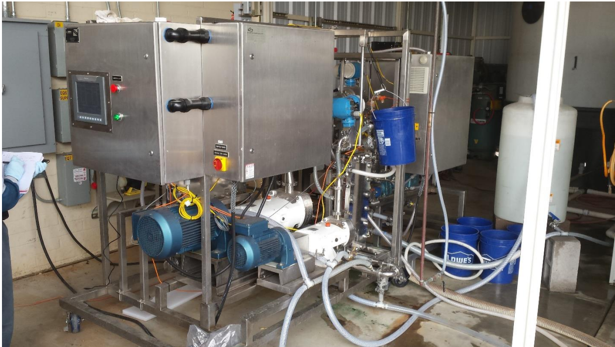
Figure 1. Photo of the Phase II continuous flow pilot scale algae dewatering skid
