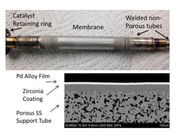
These membrane tubes have been demonstrated for hydrogen production in a bench-scale integrated water gas shift (WGS) membrane reactor process suitable for a coal-derived synthesis gas environment with nearly complete conversion of carbon monoxide in syngas and high purity hydrogen production. Large scale membrane modules may be fabricated for membrane reactor-based power generation as shown in the schematic process flow diagram.
