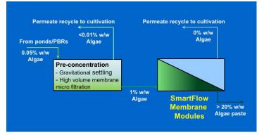
This process has been demonstrated at pilot scale with 100 L/ hr feed rate of 1% w/w algae of various strains of industrial interest producing >20% w/w algae paste in a continuous membrane filtration process. Depending on algae species we will select an appropriate pre-concentration process.
