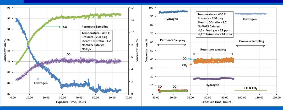
Pd-Au Binary Alloy MembranePd-A-B Ternary Alloy MembraneFeed Syngas Composition –  $H_2$  – 33%, CO – 45%, CO $_2$  – 17%, Ar – 5%,  $H_2$ S- 21 PPM
