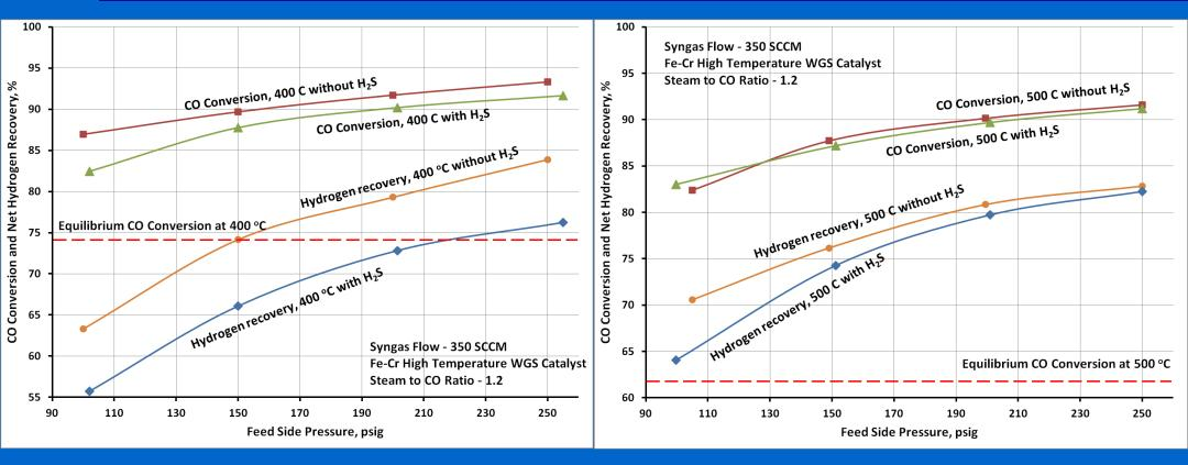
Effect of H<sub>2</sub>S on membrane performance is small at 400 °C and minimal at 500 °C
